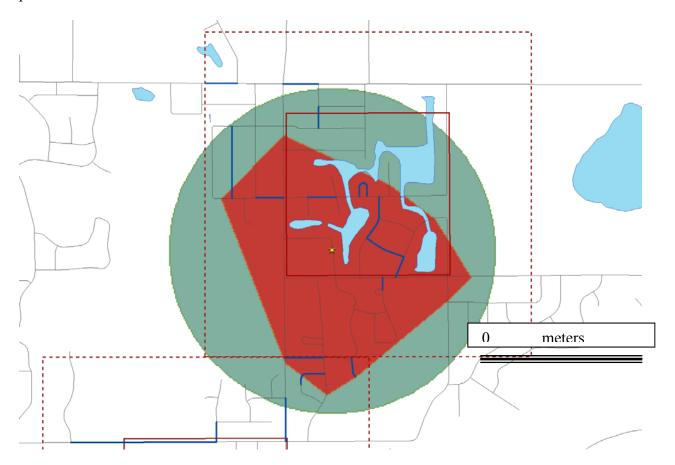
Fig. 2.5. Straight-line versus network buffers for a radius of 0.5 miles/805 meters around a hypothetical individual.
