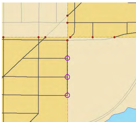
Fig. 6.5. The three purple circles identify points that should be included in the analysis, since they provide significant access to the site, are not because the road centerlines lie just inside the site boundary and do not intersect it.
