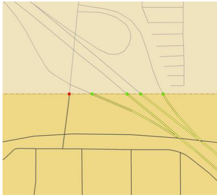
Fig. 6.2. Access points are points of intersection between road centerlines and site boundaries excluding points resulting from the intersections of site boundaries with Interstates, on- and off-ramps, and other limited access highways.
